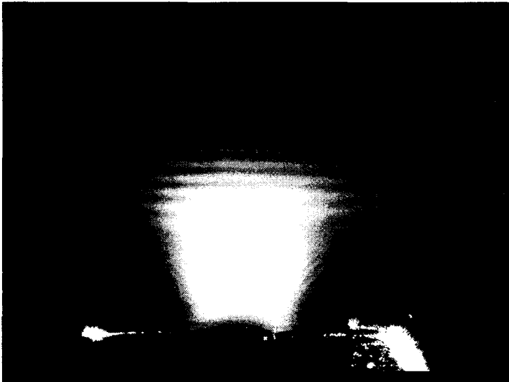
Fig. 2. The plasma in the Xe gas injected with pressure of 12 bar and irradiated by laser with energy of 900 mJ. This image was taken at 1 ns after the plasma was produced.
