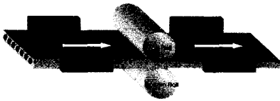
Fig. 2 Schematic diagram of cold rolling.
