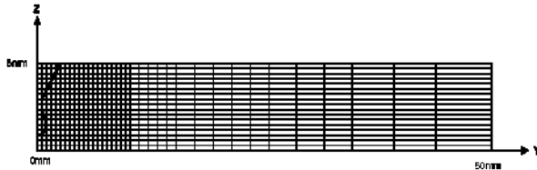
Fig.10 Schematic mesh division (two-dimensional half model).
