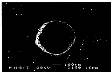
c) Laser drilling(moving on)
