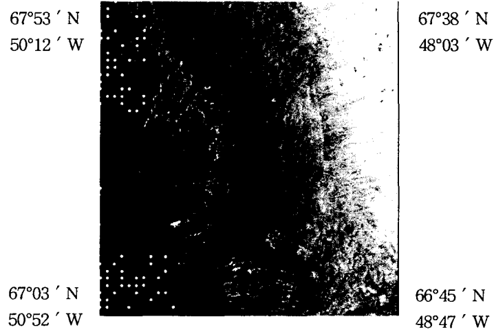
Fig. 1. SAR amplitude image of Sondrestrom area, acquired on 25 November, 1991. The white dots indicate the location of tie points used to estimate the baseline
