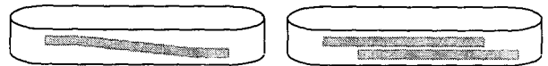
Fig. 1. The two ways of pancake winding. (a) inclined wire, (b) soldered wire.
