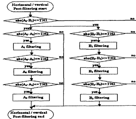
Figure 4. IIR low pass filtering in the horizontal direction
