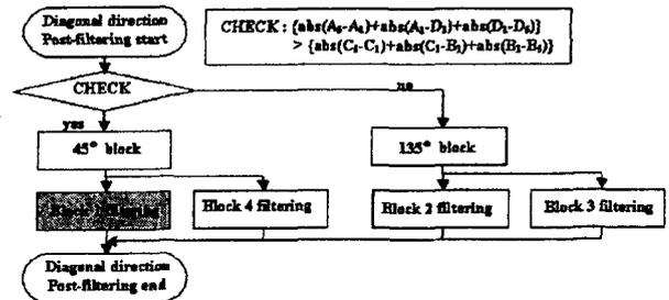
(a) The filtering procedure for diagonal direction.
