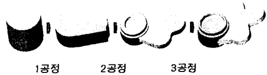
Fig. 4 Forging procedure of ball-joint socket
