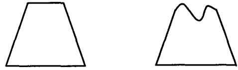
(a) Calculation shape (b) The actual shape of tooth
