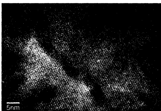
Fig. 6. The \langle 001 \rangle HRTEM images showing the distribution of all three types of precipitates in PbTe-2.5HgTe alloy aged for 300 hours at 300°C.
