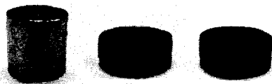
a) Specimen b) Non-annealed c) Annealed (520℃, holding time 30min, cooling in furnace)
