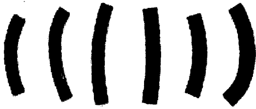
Fig. 9 A view of results of the products of curved rectangular tubes that can be manufactured by the extrusion bending process
