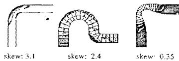
Figure 3: Diagrams to the left show corner designs examined using two dimensional field solutions. The skew normalized by the channel width is shown below each design.
