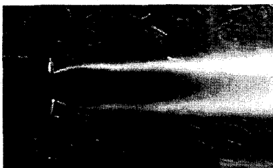
Fig. 2 Ellipsoidal Steam Jet (Nozzle ID : 10.15 mm, Steam Mass Flux : 825 kg/m 2 -s, Pool Temp. : 55 °C)
