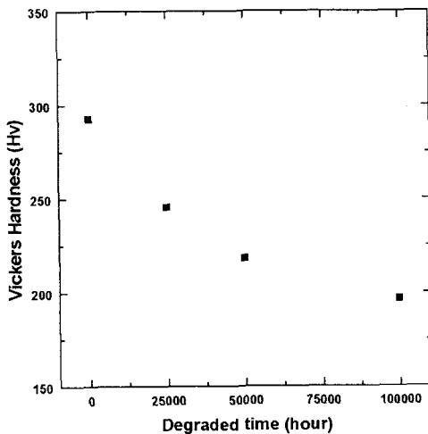
Fig. 6 Effect of degraded time on Vickers hardness
