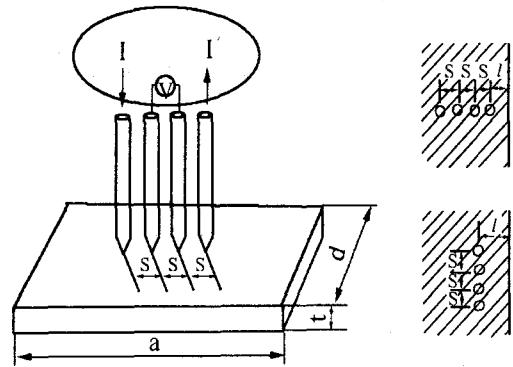
Fig. 1 Configuration of specimen boundary and 4 point probe
