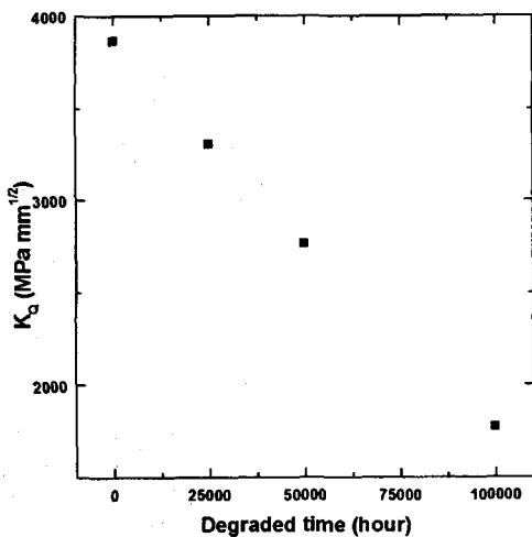
Fig. 7 Effect of degraded time on fracture toughness
