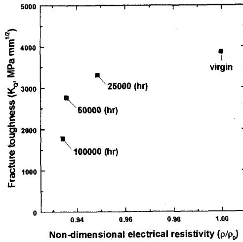
Fig. 10 Relation between fracture toughness and electrical resistivity
