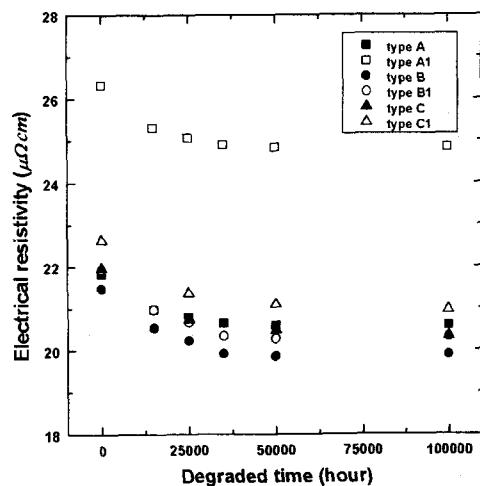
Fig. 3 Effect of degraded time on electrical resistivity
