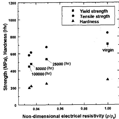
Fig. 9 Relation between material properties and electrical resistivity
