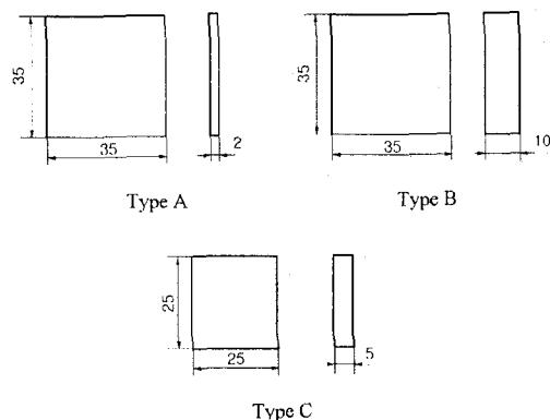
**Fig. 2** Shape and dimensions of specimens for electrical resistivity test (unit: mm)
