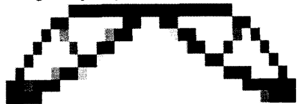
(a) Optimal topology for the specified eigenfrequency as 1 st frequency 123Hz
