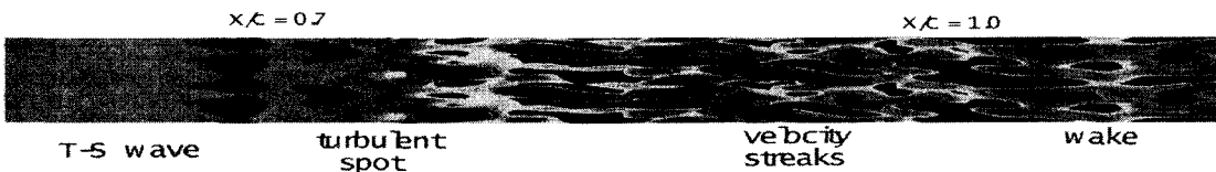
Figure 7. U-velocity fluctuation contour along the airfoil surface at Re = 7.5 \times 10^5
