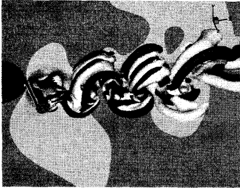
Figure 3. Streamwise vorticity contour: \omega_x = \pm 0.3 at t = 65
