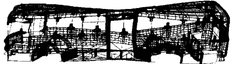
Fig. 2.1 1st torsion mode of bus B.I.W. model (16.42Hz)
