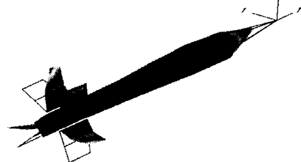
Fig. 19 2 nd Tail Wing Mode( f=49.8 Hz)
