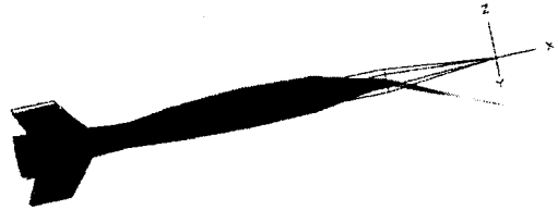
Fig. 17 Z-axis 1 st Bending Mode( f=20 Hz)
