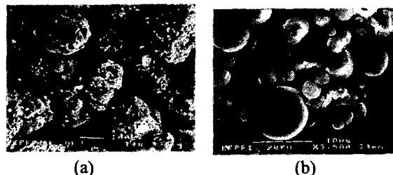
Fig. 2. SEM picture of a) +200mesh particles of the fly ash, b) -200mesh particles of the fly ash
