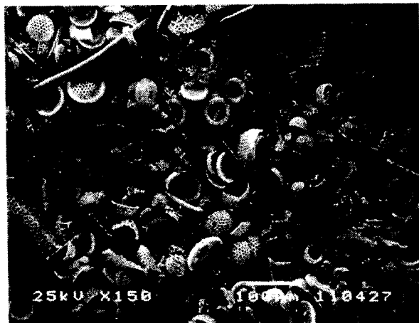
Fig. 6 Recovered diatom skeleton as over size after sieving the particles shown in Fig.5.
