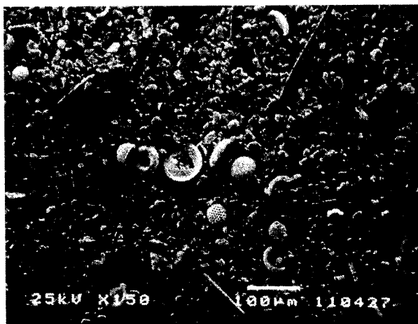
Fig. 5 Example of recovered particles in apex chamber of No.5 cyclone.
