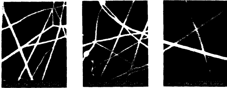
Fig. 2. SEM of PLGA fibers electrospun from an 12wt% solution in methylene chloride.
