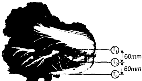
Fig. 2 Position of temperature measurement
