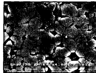
Fig. 4. Microstructure of Ni-Zn ferrite sintered at 1200°C with 1wt% V_2O_5
