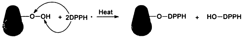
Fig. 3. Diagram of peroxide group decomposition and peroxide group and DPPH reaction.
