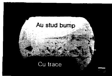
그림 1. Backscattered electron images of cross section around the solder joints.
