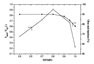
Figure Nanofiltration membrane performance (flux ratio of methanol and water and rejection of oleic acid) prepared from MPD/PIP blended amines.
