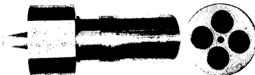
Fig. 3 The figure of rectangular conical plug and multihole container with no difference of hole diameter
