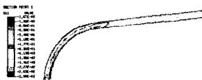
Fig. 4(b) Longitudinal stress ( \sigma_1 ) distribution with tensile pulling force that induces the average tensile stress equivalent to 20% of the yield stress after spring back
