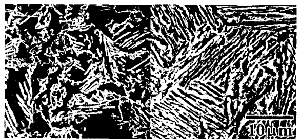
Fig. 1 SEM micrographs showing the morphology and distribution of secondary phases ; (a) 800/325°C (T80-3) and (b) 950/425°C (T95-3)
