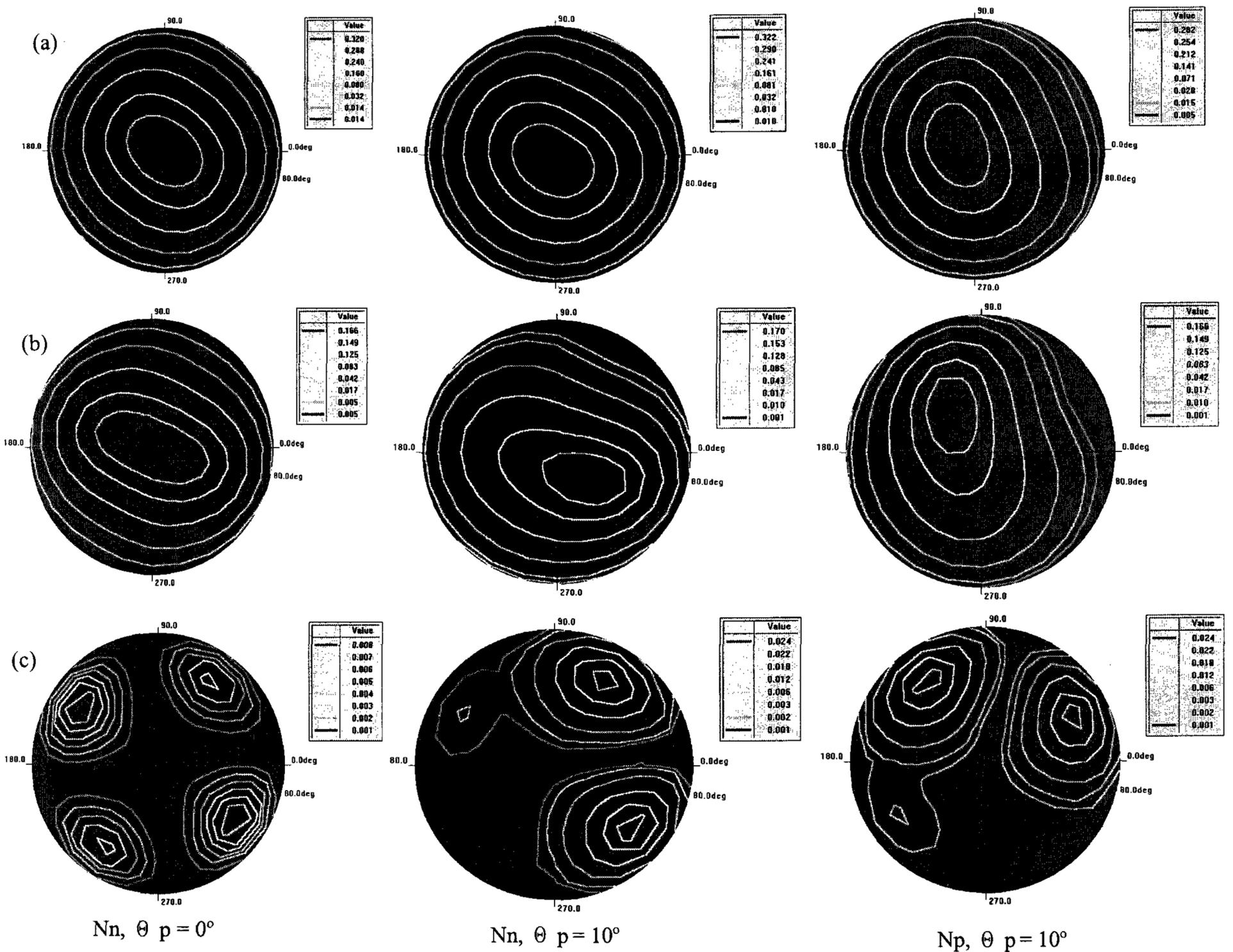
Fig. 1 Iso-luminance contours for (a) bright, (b) grey, (c) dark states as a function of pretilt angle and LC type.
