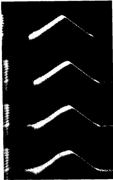
Fig.6 Visualized particle motions behind a porous fence of \epsilon=20\% at U_0=V_{c,30\%} .
