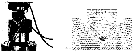
Fig. 3 Assembly of jig, specimen, block for test and two dimension model for FEM
