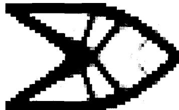
Fig. 12 Optimization result using classical artificial material model (no penalty and no postprocessing)
