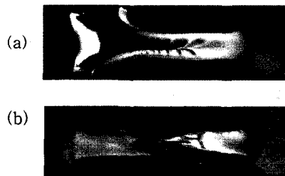
Fig.12 Schematic diagram of failure plane for the radius of notch tip at -30^{\circ}\text{C} , 0^{\circ}\text{C} , 20^{\circ}\text{C}
