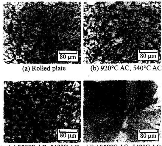
Fig. 2 Optical micrographs of heat treated Ti-6Al-4V alloy
