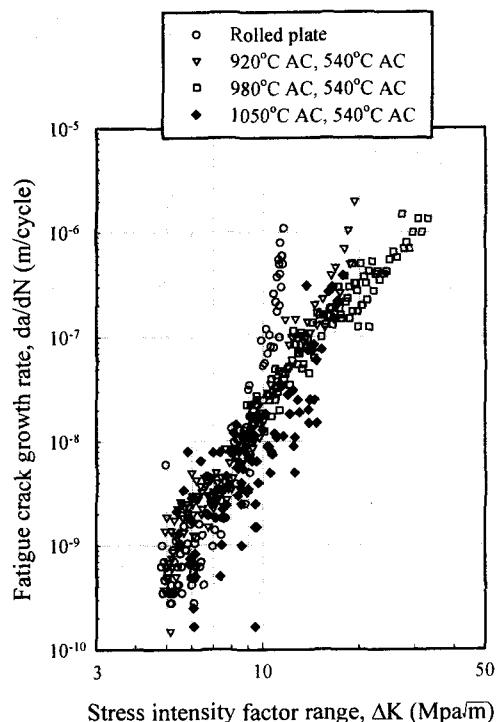
Fig. 6 Relationship between fatigue crack growth rate,  $da/dN$  and stress intensity factor range,  $\Delta K$
