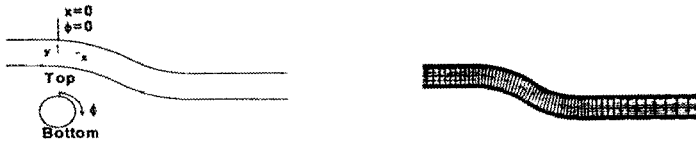
Fig. 1. Geometry and grid system for circular S-duct(77x33x49)
