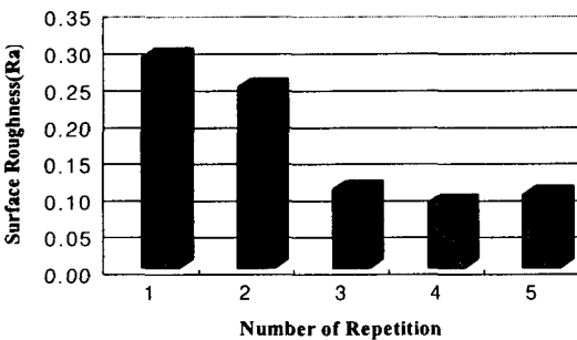
Fig. 10 Change of surface roughness in traverse grinding process
