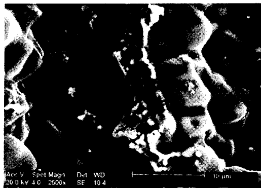
Fig.2 SEM microfractographs of solidification crack
