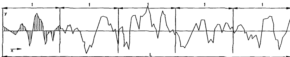
Fig. 4. Profile of a curved line for centerline average height roughness designation method.
