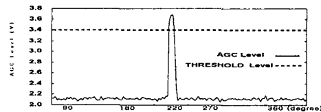
Fig. 3 The observed AGC signal level from BS tuner
