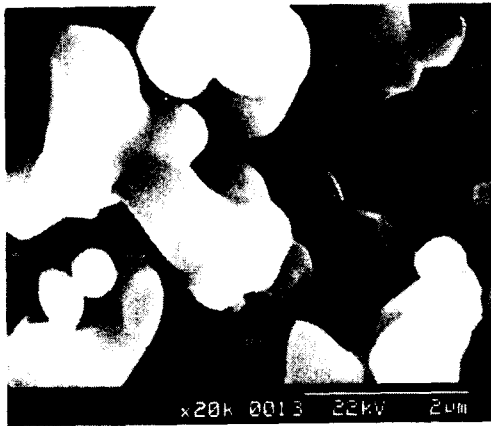
Fig. 7. SEM of Ni_{0.5}Mn_{0.1}Zn_{0.4} \cdot Fe_2O_4 Heat-Treated at 1200 °C
