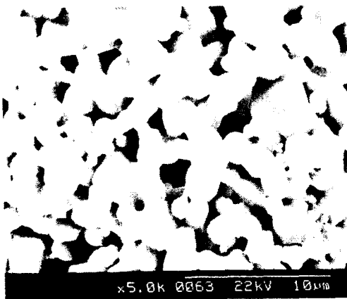
Fig. 8. SEM of Ni_{0.5}Mn_{0.1}Zn_{0.4} \cdot Fe_2O_4 Heat-Treated at 1300 °C
