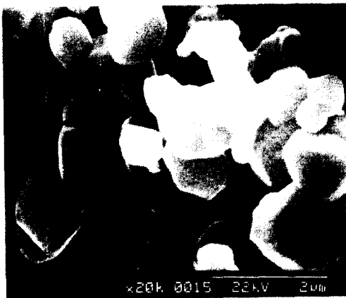
Fig. 9. SEM of Ni_{0.5}Mg_{0.1}Zn_{0.4} \cdot Fe_2O_4 Heat-Treated at 1200 °C
