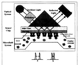
Fig 1. Schematic diagram of protein chip system. Protein chip system consists of optical (detection) system, sensor chip and microflid system. Binding of biomolecules on the surface of sensor chip causes the shift of SPR angle (see
