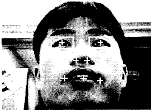
Fig. 4 Result of face tracking - Two rectangles are rough eye regions. The crosses are eyes, nostrils, and mouth center/corners
