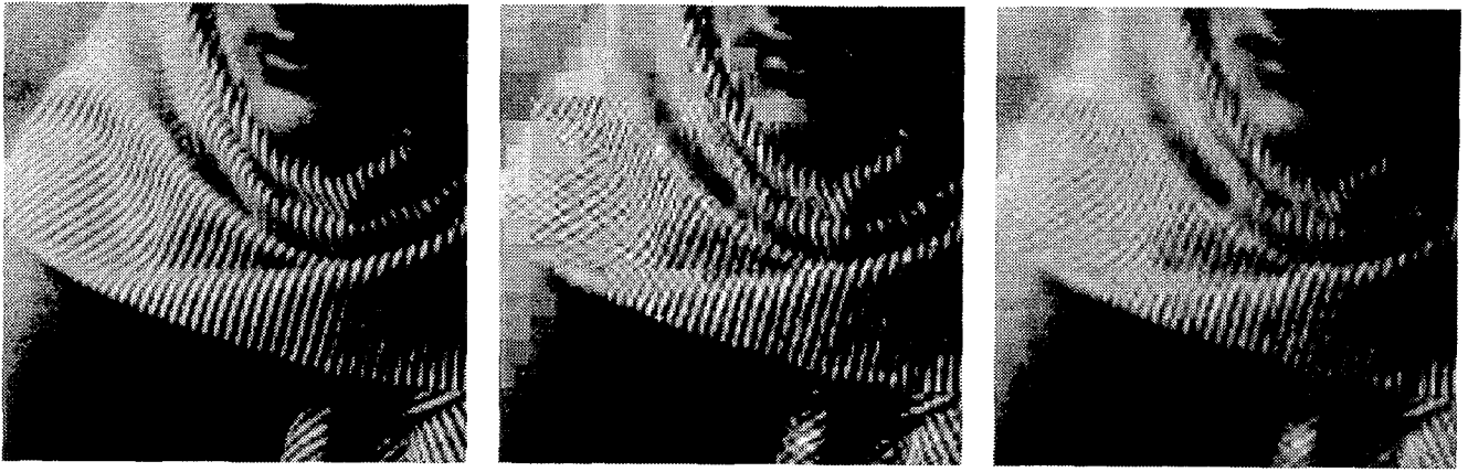
Figure 5: The original 512 \times 512 'Barbara' (left), its compressed version at 0.30 bpp (center), and the deblocked image with the proposed iterative algorithm for three iterations (right).
