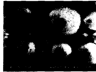
Fig. 1 The SEM image of 3Y-PSZ powder made by spray drying methods.
