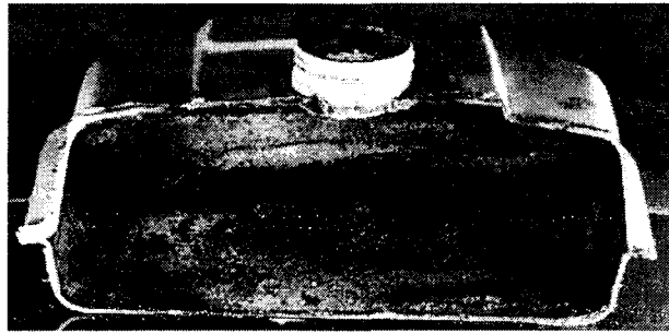
Fig 4. Cross section view of fuel tank in cultivator
