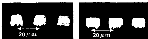
Subtractive Semi-additive Fig.5 Cross view of line
