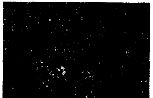
Fig. 5(c). Photograph of workpiece according to grit size(SiC, #240, 4.0 \mu mRa, 20X)
