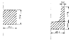
Fig. 3 Shape and Dimension of Preform and Product
